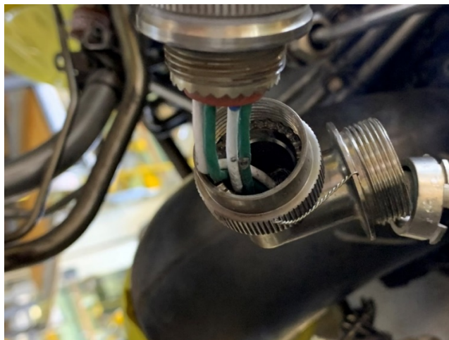
Image 3 – J10-B, Wire 98 Chaffing, exposed wire causing intermittent connectivity
