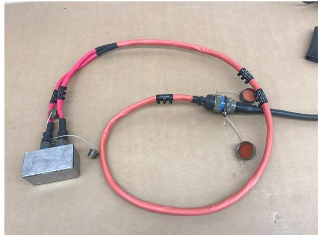
AWTS Cockpit Control Thrust Drive Actuator Cable P/N: 18D5371-1
