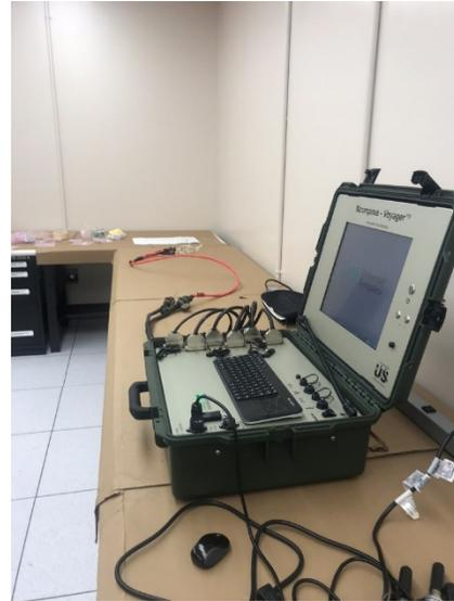
AWTS Rudder Cable connected to Voyager via AWTS Patch Cable
