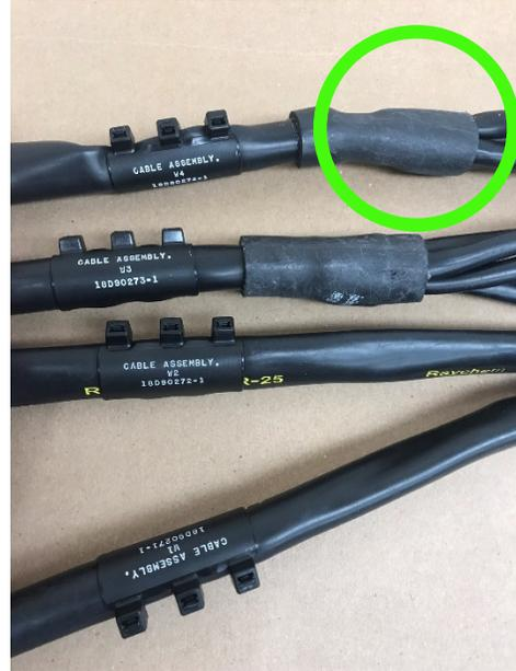
Intermittence was detected and isolated in the cable splice of W4
