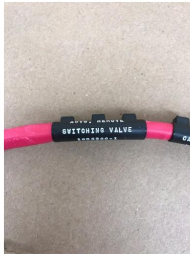
AWTS Remote Switching Valve Cable P/N: 18D5386-1
