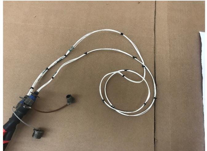
V-22 modified Rudder Actuator Cable
