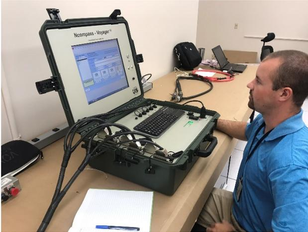
Advanced Technology Team Engineer utilizing Voyager to test AWTS V-22 CCFDA Cables
