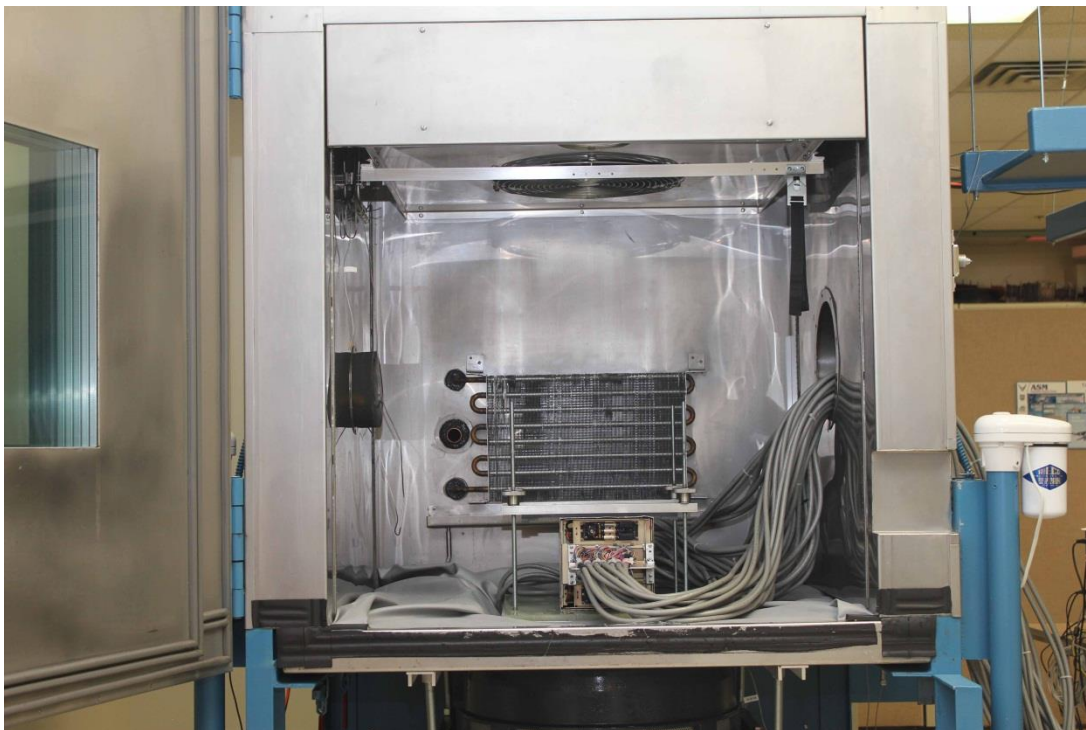
ELAC mounted for testing in the IFDIS environmental chamber
