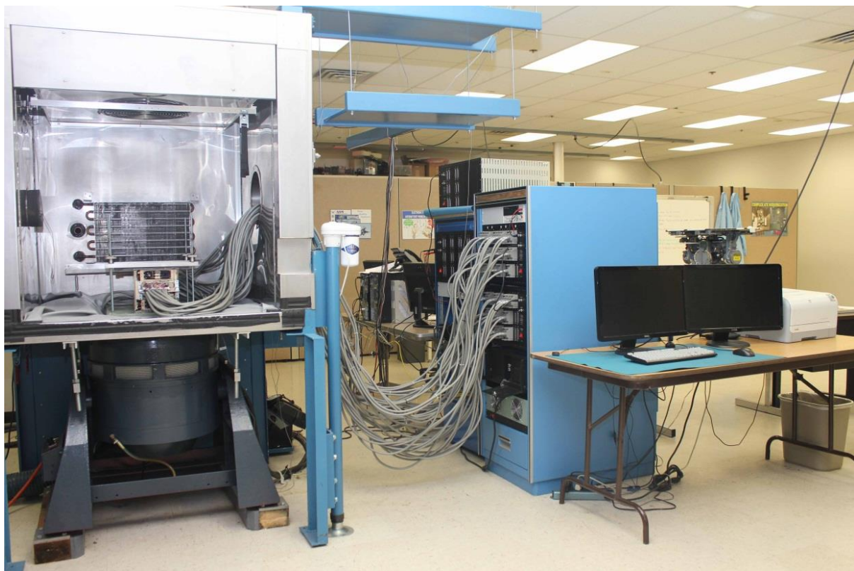
ELAC on the shaker in the environmental chamber connected to the IFD through the ITA
