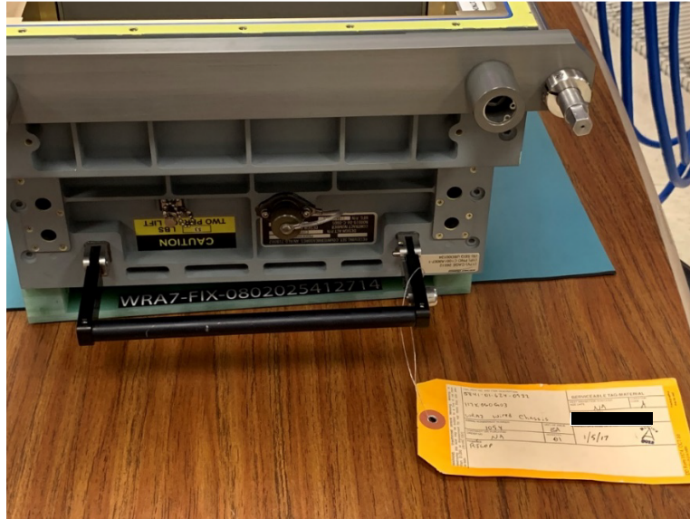
Photo A - WRA 7 with Service Tag Condition Code A
