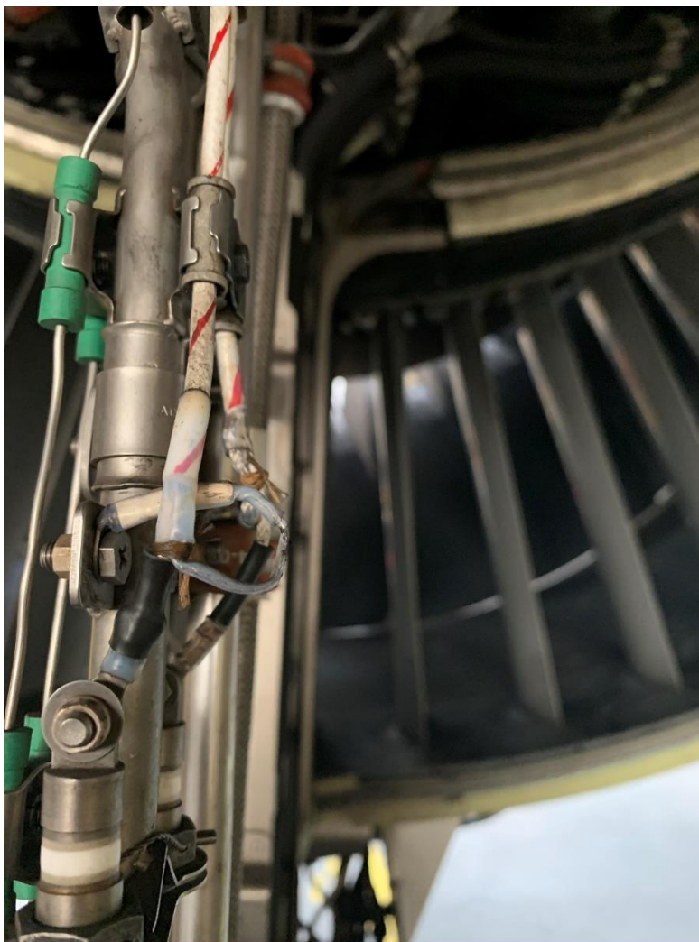
Graphic 9 – Wire Assembly installed on GE90 Engine – excessive wire bend prone to degradation and intermittence
