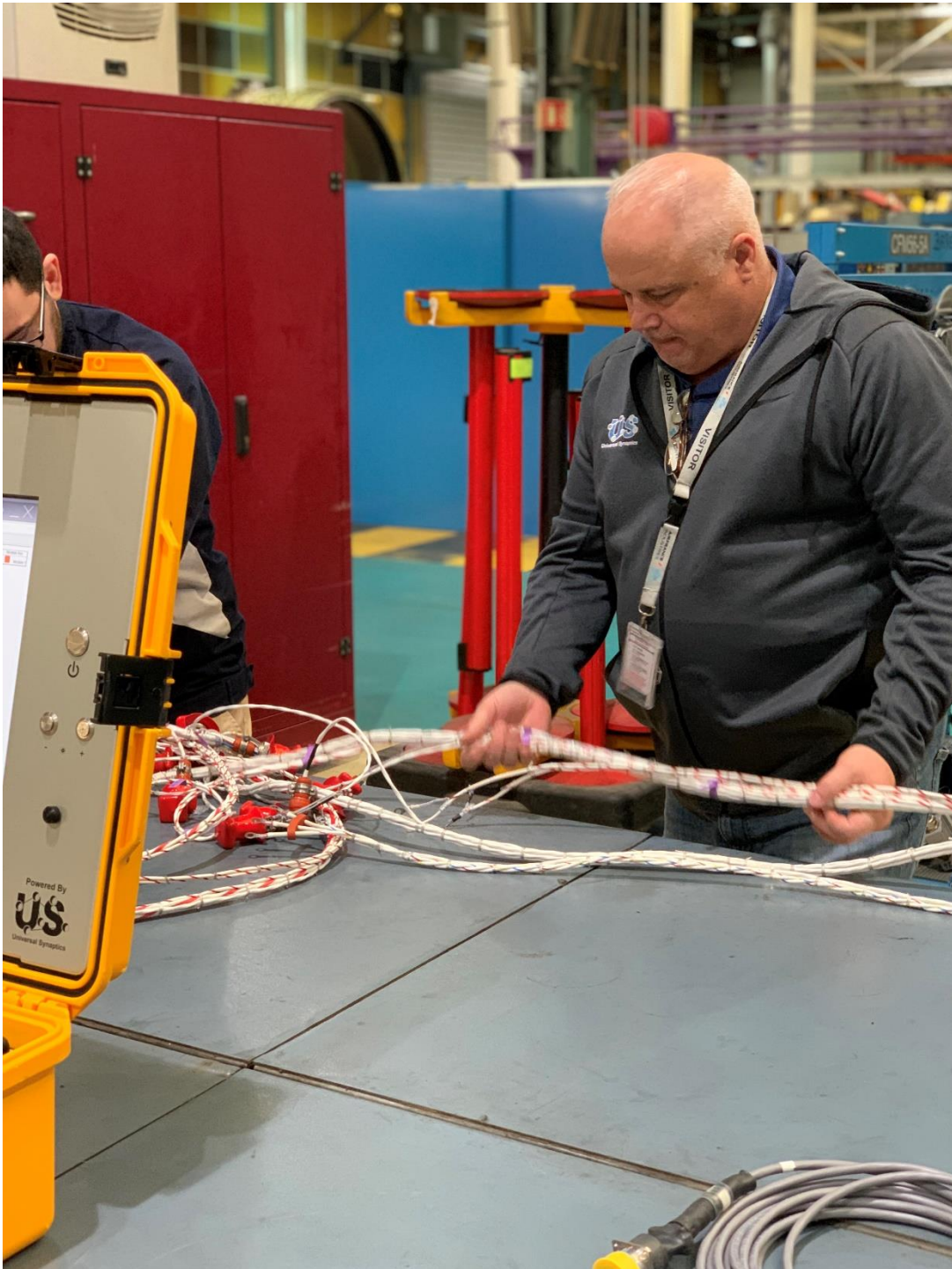
Graphic 11 – USC Technical Director connecting Wire Bundle Assembly to IFD interface test adapter (ITA)
