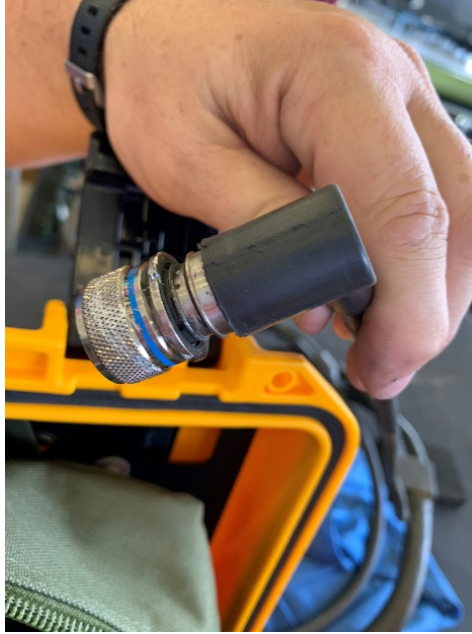
Right (Cable ID: W186) Lock Ring Overtightened
