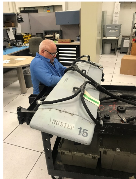
Technician connecting PATS-70 cable to DRA
