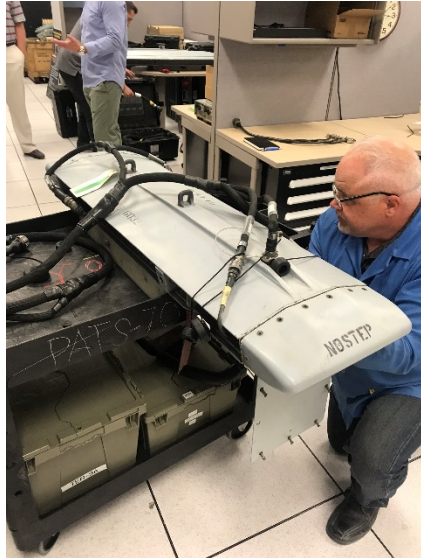
Technician connecting PATS-70 cable to DRA
