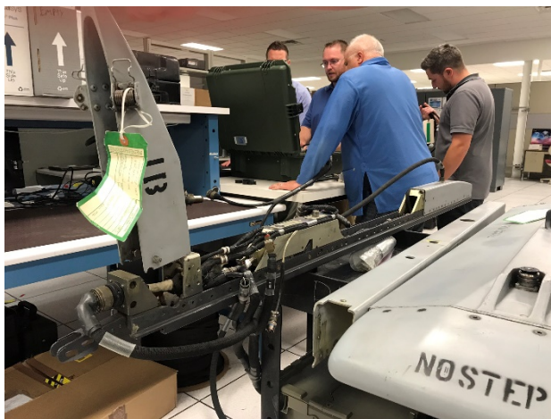
Voyager connected to LAU via PATS-70 cable
