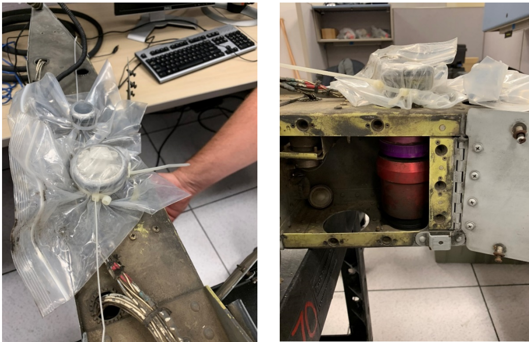
A-10 Pylon #6 Fuel Tank Plumbing
