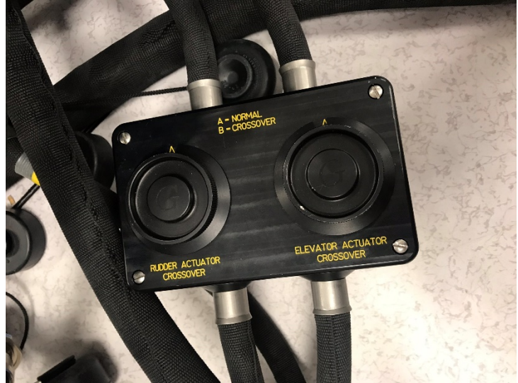
SAS Umbilical Rudder Actuator Crossover and Elevator Actuator Crossover
